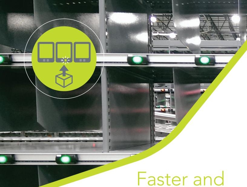
The LP Put solution optimizes batch picking and high-speed sortation operations with a process sometimes called pick-to-light in reverse. With put-to-light, operators scan an item and the locations representing a store or customer needing that item illuminate. From straight forward scan-and-put workstations and put walls, to more complex sortation applications, LP Put offers options that maximize speed and accuracy.
