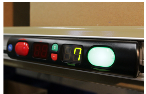
MW2040PRG-22: 2x2-Digit Display, Red/Green Domed Light/Confirm Button LED for Dual Location Applications
